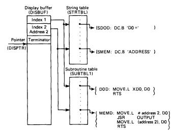
Figure 4. Display buffer (DISBUF) initialized with two conditions: the processor register (D0) and a memory location
