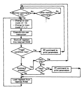
Figure 7. Flowchart of the conditional trace process
