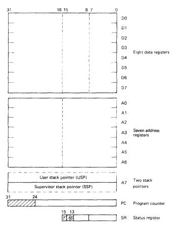
Figure 1. MC68000 programming model
