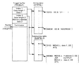
Figure 5. Trigger buffer (TRGBUF) initialized with two conditions: the processor register (D1) and a memory location
