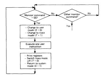
Figure 2. Flowchart of the single-step process
